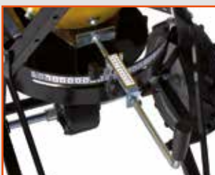
Gate opening control
