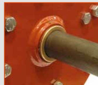
Both hub flanges are welded and equipped with two bronze bushings per rotor
