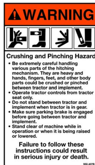
Fig. 2 - Safety decals - implement; replace immediately if damaged.
