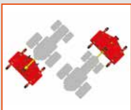
Reversible three point hitch for front or rear tractor mounting
