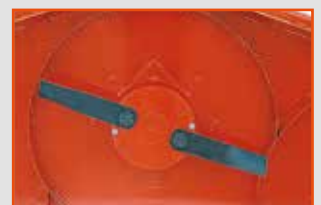
Rotor with free swinging blades
