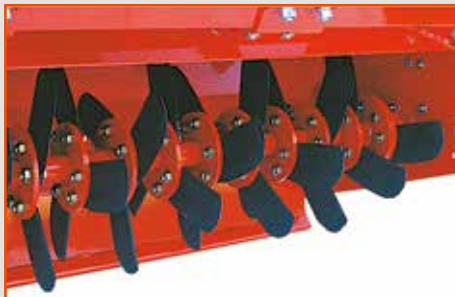
Aerator rotor with straight blades with 2-1/8" flange spacing
