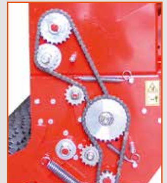
Seed distribution engaged by ASA 50 chain transmission
