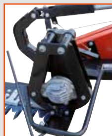
Cast aluminium connecting rods with cooling fins
