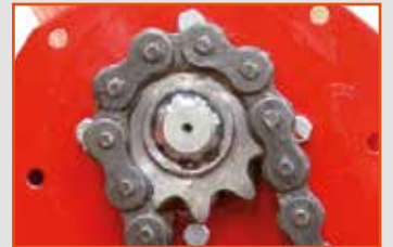
Lateral ASA 100 chain drive transmission in oil bath
