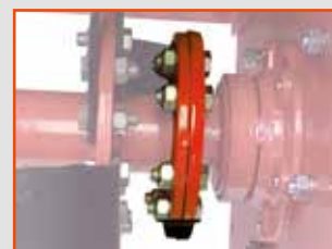
Rotor shaft with flanges for easy blade replacement
