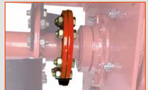
Rotor shaft with flanges for easy blade replacement
