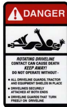
placed on outer shield
